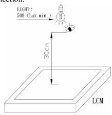
The inspection area of LCD panel shall be within the range of following limits.
